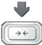
Press and release the **Join** button on the side of the SUB. The indicator flashes green and white while the SUB is connecting
