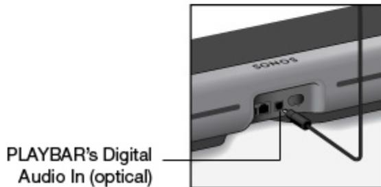
**IMPORTANT:** Be sure to remove the protective caps from each end of the supplied optical audio cable before inserting.
